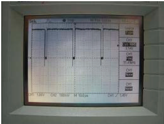
U9 Pin 1 –DAC_HS (OSD On), 15.72kHz
